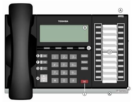
20 Programmable Feature Buttons 4-Line LCD Telephone
